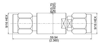
Note: (1)Re commend coupling nut torque: 13 in.-lbs.
