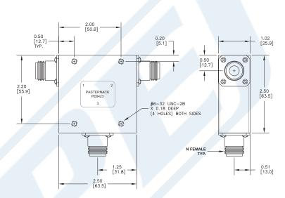
50 Ohm N Circulator Operating From 380 MHz to 460 MHz And 1000 Watts With 20 dB Isolation from Pasternack Enterprises has same day shipment for domestic and International orders. Our RF, microwave and fiber optic products maintain a 99% availability and are part of the broadest selection in the industry.
