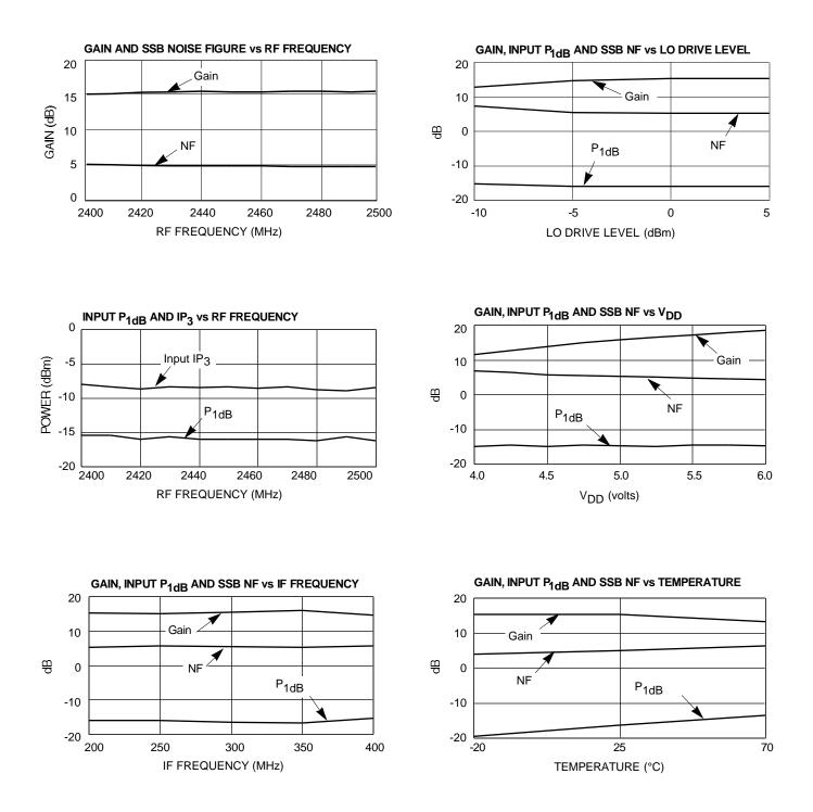
1. Test conditions (unless otherwise specified): RF = 2450 MHz, IF = 200 MHz, LO = 2250 MHz, 0 dBm,  $V_{DD}$  = +5 V,  $V_{GG}$  = -5 V,  $T_A$  = +25°C
