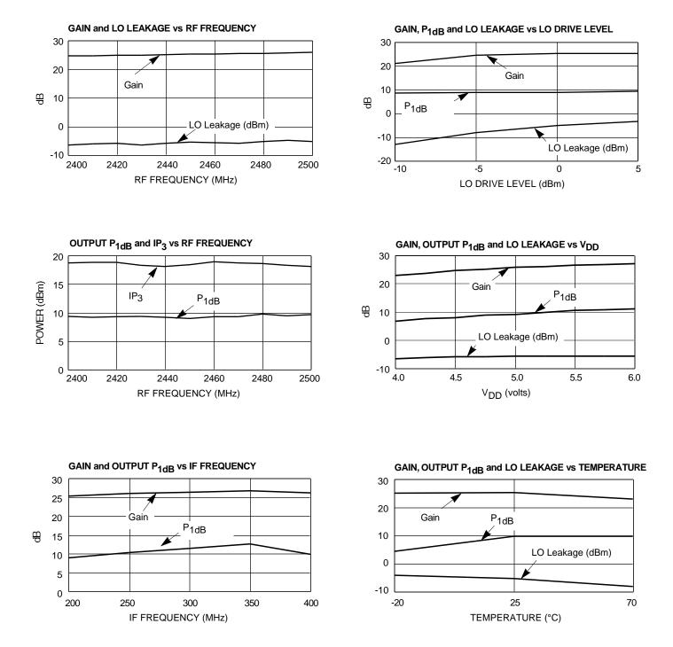
1. Test conditions (unless otherwise specified): RF = 2450 MHz, IF = 200 MHz, LO = 2250 MHz, 0 dBm,  $V_{DD}$  = +5 V,  $V_{GG}$  = -5 V,  $T_A$  = +25°C
