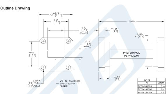
WR-42 Instrumentation Grade Straight Waveguide Section 9 Inch Length with UG595/U Flange Operating from 18 GHz to 26.5 GHz from Pasternack Enterprises has same day shipment for domestic and International orders. Our RF, microwave and millimeter wave products maintain a 99% availability and are part of the broadest selection in the industry.
