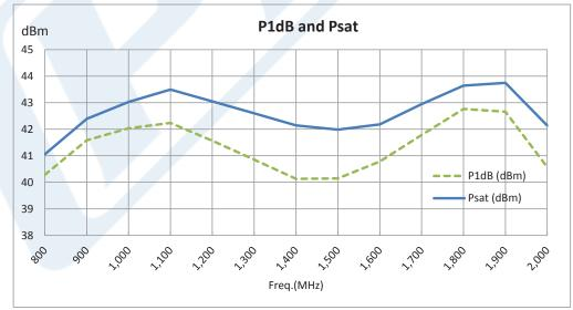
Click the following link (or enter part number in "SEARCH" on website) to obtain additional part information including price, inventory and certifications: 41 dB Gain, 12 Watt Psat, 800 MHz to 2 GHz, High Power High Gain Amplifier, 50 dBm IP3, SMA PE15A5035
