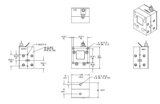
Q-Band (B-Band, WR-22) Low Noise Power Amplifier (Outline is also valid for Ka-Band, WR-28.)
