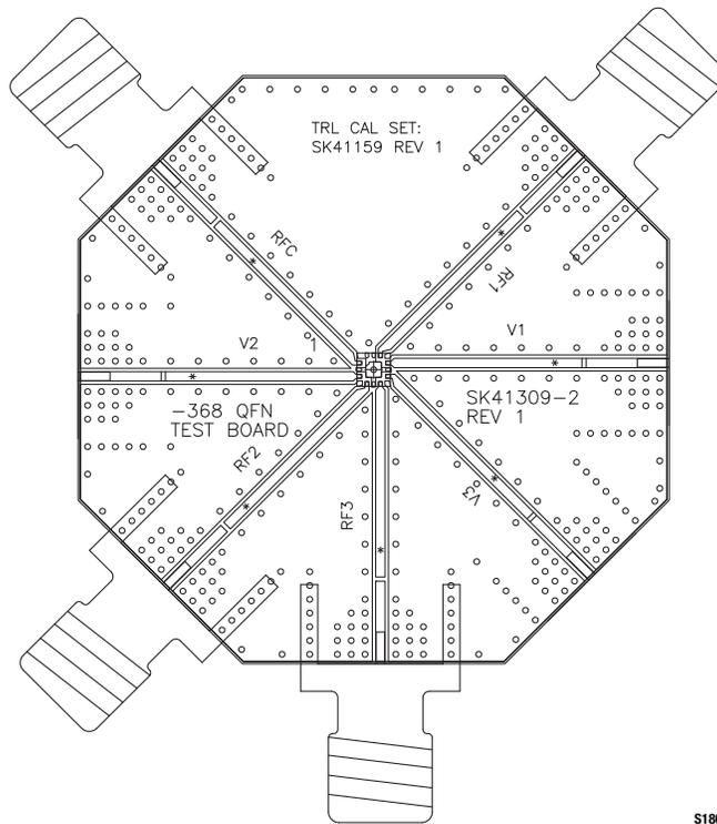
Figure 13. SKY13346-368LF Evaluation Board Assembly Diagram
