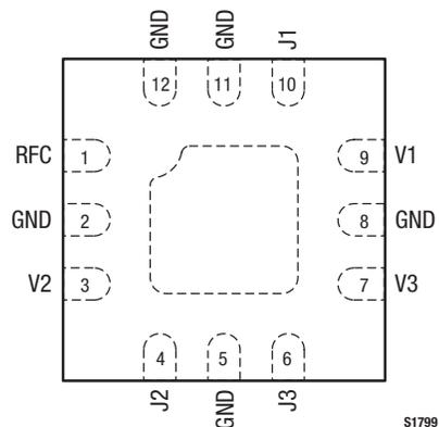
**Figure 2. SKY13346-368LF Pinout – 12-Pin QFN (Top View)**
