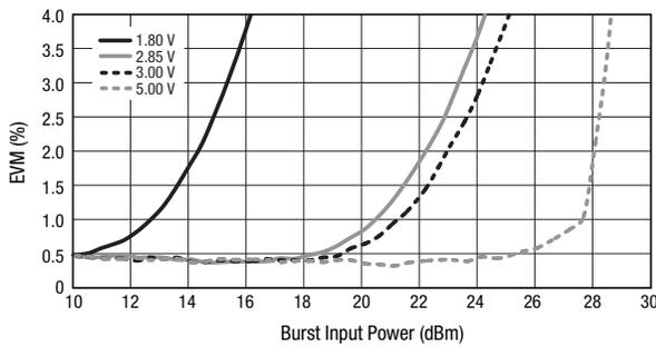
Figure 11. EVM vs Burst Input Power Over Voltage
