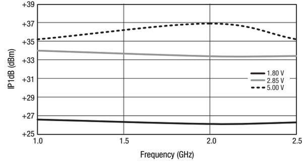
Figure 10. Input 1 dB Compression Point vs Frequency
