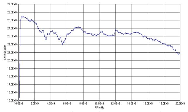
Maximum available level with options R&S®SGU-B120V, R&S®SGU-B26 (meas.) in combination with R&S®SGS100A.
