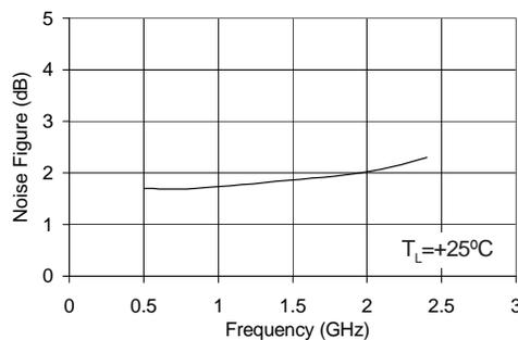
Typical RF Performance Over Temperature ( Bias:  $V_D = 3.2\text{ V}$ ,  $I_D = 45\text{ mA}$  (Typ.) )
