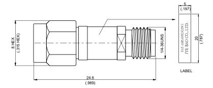
Nominal impedance:  $50\Omega + /-0.25\Omega$  over operating temperature range.
