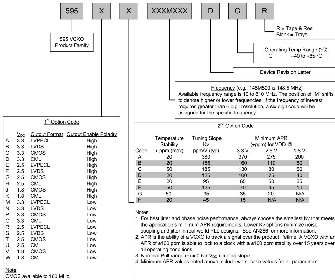
Example Part Number: 595AE148M500DGR is a 5 x 7 mm VCXO in a 6 pad package. The nominal frequency is 148.5 MHz, with a 3.3 V supply, LVPECL output, and Output Enable active high polarity. Temperature stability is specified as  $\pm 20$  ppm and the tuning slope is 95 ppm/V. The part is specified for a -40 to +85 °C ambient temperature range operation and is shipped in tape and reel format.
