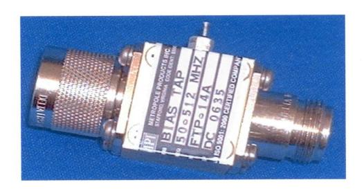
The FTP-14A Bias Tap is used to provide a DC path to one side of a 50 Ohm transmission line. An integral blocking capacitor isolates the DC from the other side of the line.
