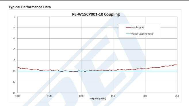
Click the following link (or enter part number in "SEARCH" on website) to obtain additional part information including price, inventory and certifications: WR-15 10 dB Directional Waveguide Coupler With UG-385/U Flange and H-Plane Coupled Port From 50 GHz to 75 GHz V Band PE-W15CP001-10
