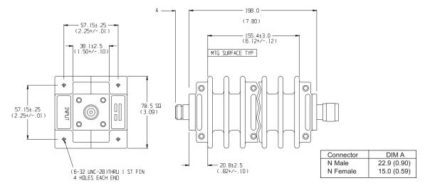
NOTE: All dimensions are given in mm (inches) and are maximum, unless otherwise specified.
