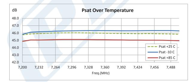
Click the following link (or enter part number in "SEARCH" on website) to obtain additional part information including price, inventory and certifications: 58 dB Gain, 15 Watt Psat, 7.2 GHz to 7.5 GHz, High Power High Gain Amplifier, GaN, SMA PE15A5019
