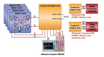
viding very fast and accurate measurements. Repeated connect / disconnect cycles for measuring PIM of DUTs in different frequency bands is a thing of the past. Both PIM and S-parameters are now measured without changing the physical connection. This results in a major reduction of overall test time and increases test throughput significantly.
