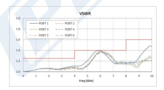
Click the following link (or enter part number in "SEARCH" on website) to obtain additional part information including price, inventory and certifications: SP6T Electromechanical Relay Normally Open Switch DC to 10 GHz, N, 160 Watts, 12V Control PE71S6194
