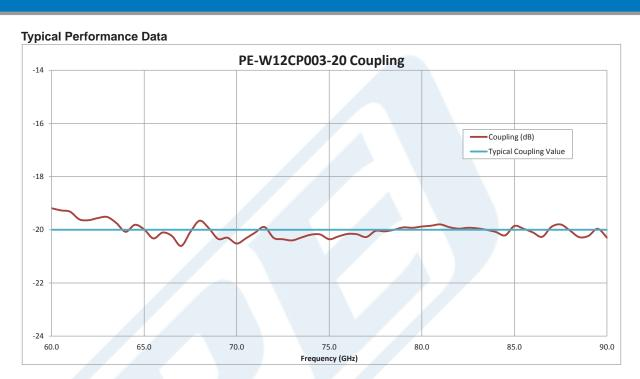
Click the following link (or enter part number in "SEARCH" on website) to obtain additional part information including price, inventory and certifications: WR-12 20 dB Directional Waveguide Coupler With UG-387/U Flange and E-Plane Coupled Port From 60 GHz to 90 GHz E Band PE-W12CP003-20
