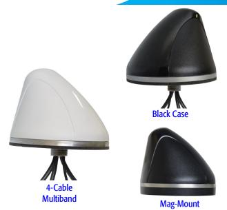
The SMW-410 Series Antennas features 4 elements in one antenna radome. The unique feature of this model is that it offers two identical high gain elements covering 2.4 GHz & 4.9-6.0 GHz. Of the remaining two elements in the SMW-410, one is used for GPS at 1575 MHz and the other covers 2.1-2.5 GHz & 4.4-6.0 GHz. All three elements offer an impressive 5 dBi gain.
