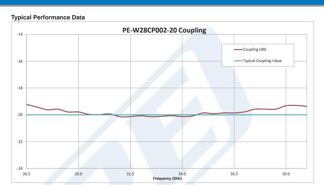
Click the following link (or enter part number in "SEARCH" on website) to obtain additional part information including price, inventory and certifications: WR-28 20 dB Directional Waveguide Coupler With UG-599/U Flange and H-Plane Coupled Port From 26.5 GHz to 40 GHz Ka Band PE-W28CP002-20
