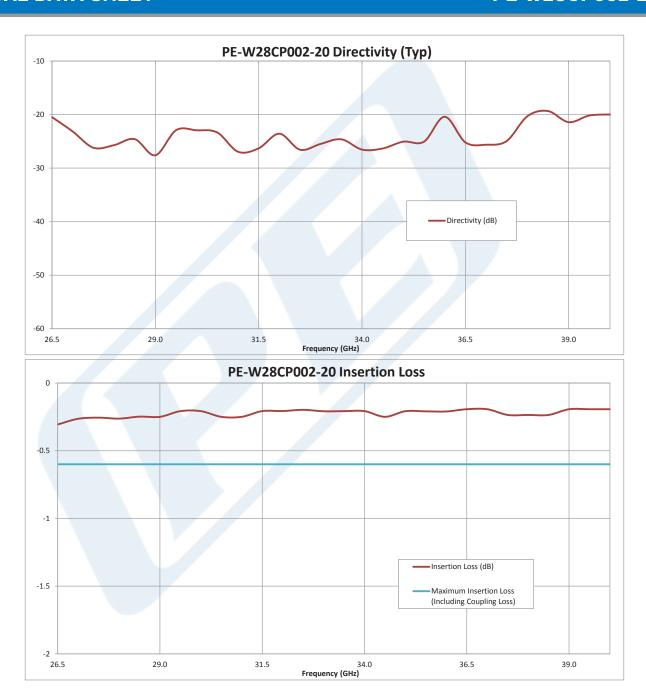
Click the following link (or enter part number in "SEARCH" on website) to obtain additional part information including price, inventory and certifications: WR-28 20 dB Directional Waveguide Coupler With UG-599/U Flange and H-Plane Coupled Port From 26.5 GHz to 40 GHz Ka Band PE-W28CP002-20
