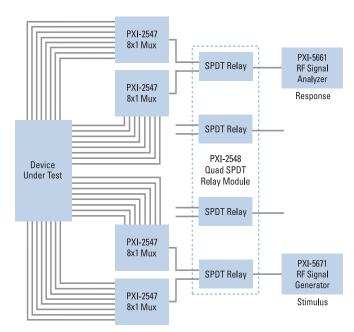
Figure 1. 16x1 Stimulus-Response Test Using PXI RF Switches
