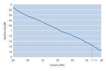
Figure 2. The insertion loss of the PXI-2547 8x1 multiplexer at its bandwidth (2.7 GHz) is only about 1.6 dB.
