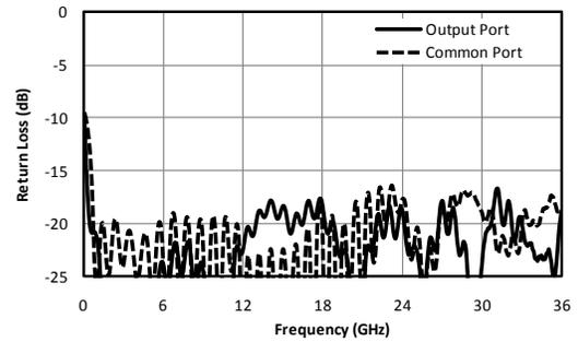
Fig. 2. Return loss for output and common ports.
