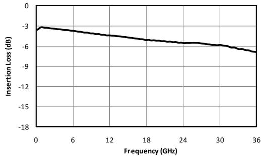
Fig. 1. Common port to output port insertion loss.
