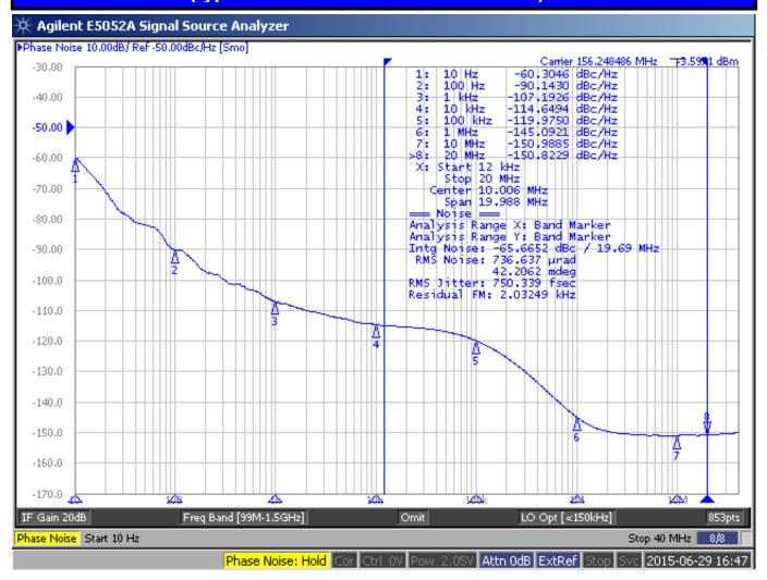
Jitter is frequency dependent. Below are typical measured values for 156.25 MHz. (Consult Fox Tech Support for other frequencies.)
