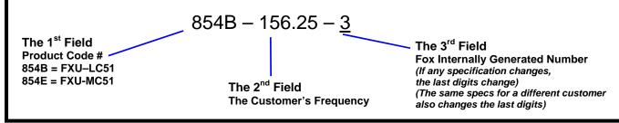
This example, FXU-LC515R-156.25 = LVDS Output, Ceramic, 5 x3.2mm Package, 1.8V, ±50 PPM Stability, -40 to +85°C Temperature Range, at 156.25 MHz
