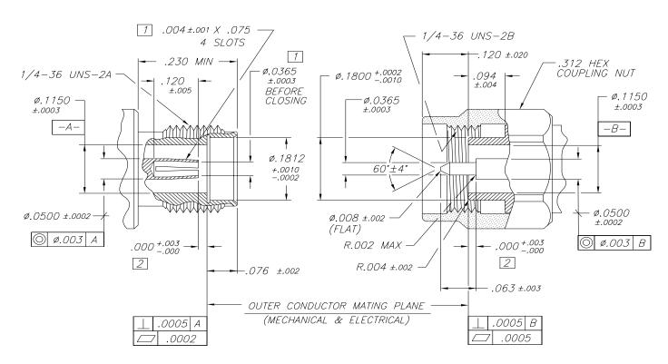
Figure 1: Female K (2.92mm) and Male K (2.92mm) Connector
