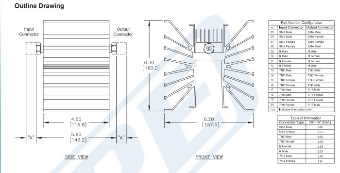
20 dB Fixed Attenuator, N Female To N Female Directional Black Aluminum Heatsink Body Rated To 300 Watts Up To 3 GHz from Pasternack Enterprises has same day shipment for domestic and International orders. Our RF, microwave and millimeter wave products maintain a 99% availability and are part of the broadest selection in the industry.
